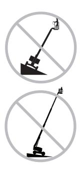
Do not raise or extend the boom unless the machine is on a firm, level surface.
