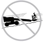
Do not operate a boom in the path of any crane unless the controls of the crane have been locked out and/or precautions have been taken to prevent any potential collision.
