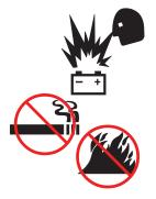
Keep sparks, flames and lighted tobacco away from batteries. Batteries emit explosive gas.
